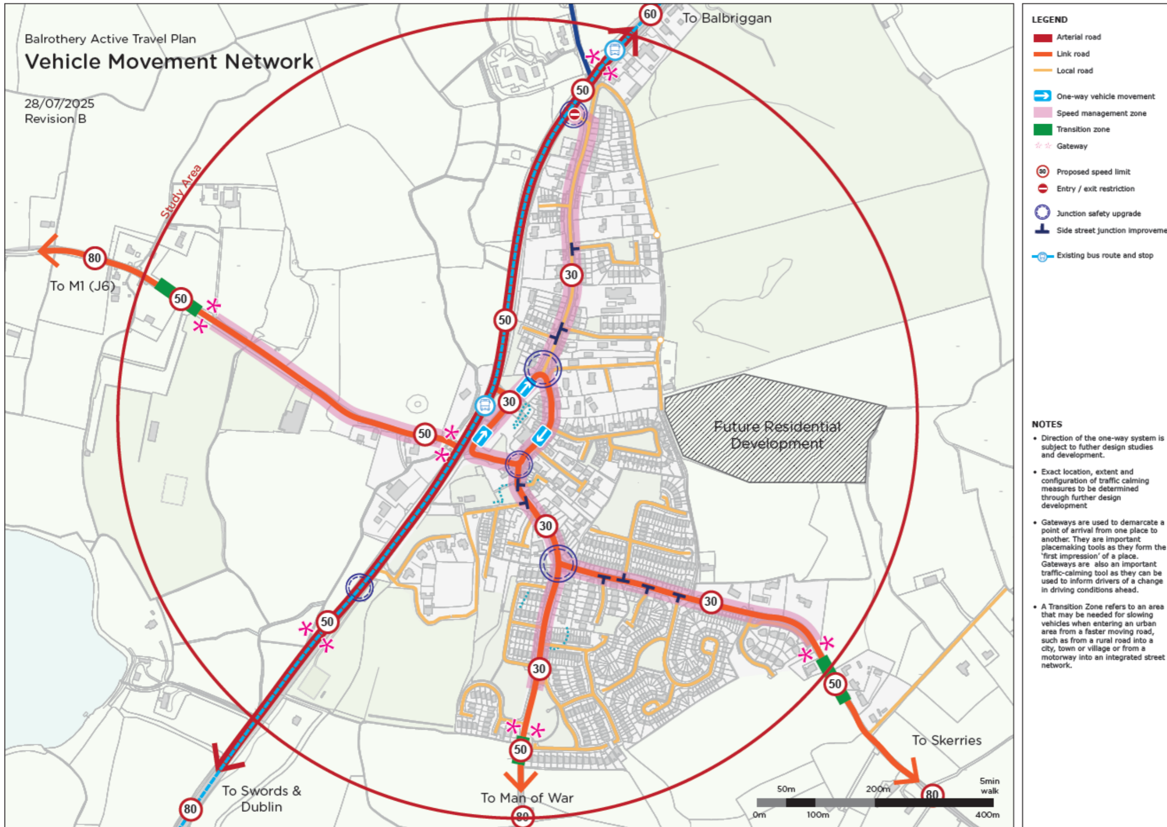
Figure 6-2: Proposed speed management and traffic movement
