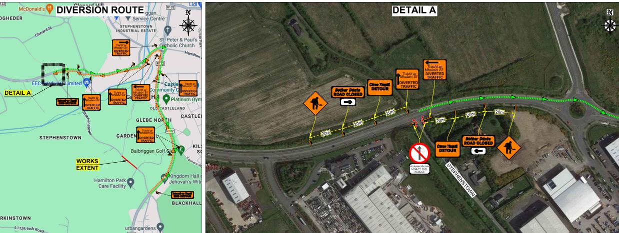
**DESIGN PARAMETERS** 1(IV) CHAPTER 8 ROAD LEVEL: SPEED LIMIT: ≤ 60km/h ROADWORKS TYPE: NUMBER OF SIGNS: SIGN VISIBILITY: 60m DISTANCE BETWEEN SIGNS: 20m SIGNS SIZE RECTANGULAR - MIN. 600mm SIGNS SIZE CIRCULAR - MIN.: 600mm CONE HEIGHT - MIN. 750mm TAPER CONE SPACING: N/A ONGITUDINAL CONE SPACING: N/A RATE OF TAPER: N/A N/A SAFETY ZONE: JNOBSTRUCTED WIDTH: N/A MAXIMUM LENGTH OF SHUTTLE: N/A MINIMUM LANE WIDTH: N/A ROAD CLOSURE TM SYSTEM:
