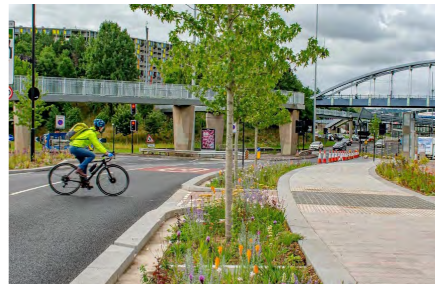
Fig. 9-12: Example of Rain Garden along Road / Path
