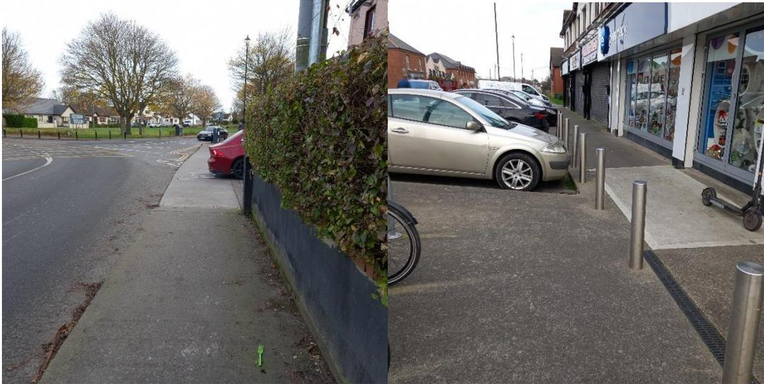
Perpendicular parking with inadequate widths for car overhang can cause damage to existing posts and signs.
