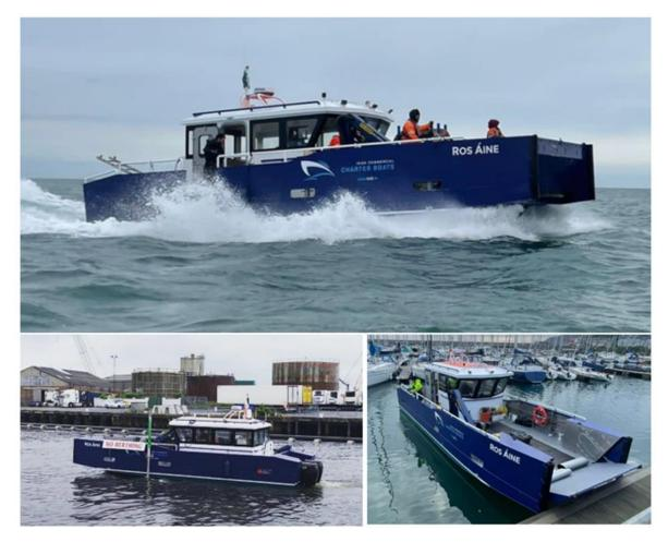
Ros Áine (LOA 12m, beam 4m and draft 0.8m) is a shallow drafted catamaran. The vessel colour is blue. The vessel will operate on a 6hr basis working out of Malahide Marina and will display appropriate day shapes & lights during survey operations.
