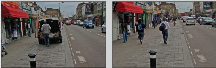
Image 43: Example from Walworth Road, London, where a loading bay provided within a verge, can revert to pedestrian space when not used. Source: DMURS.
