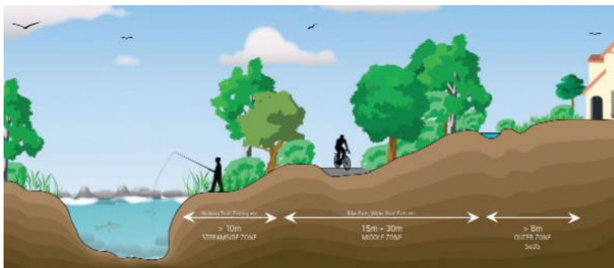
Diagram illustrating riparian buffer sub zones (from IFI guidance document - Planning for watercourses in the urban environment - http://www.fisheriesireland.ie/Download-document/86-Planning-for-Watercourses-in-the-Urban-Environment.html )
