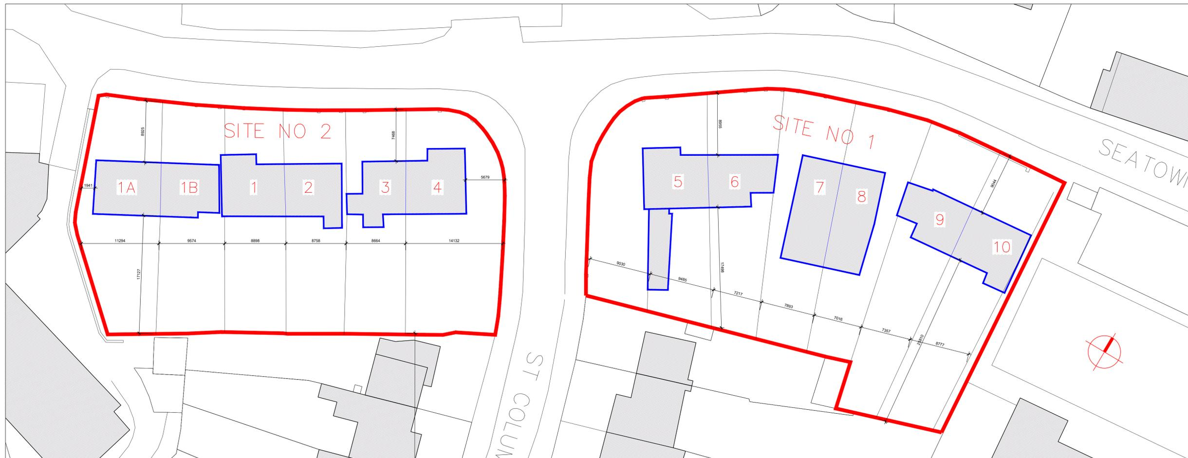
SITE PLAN NO 1 & 2 INDICATING DEMOLITIONS (SCALE 1:250)
