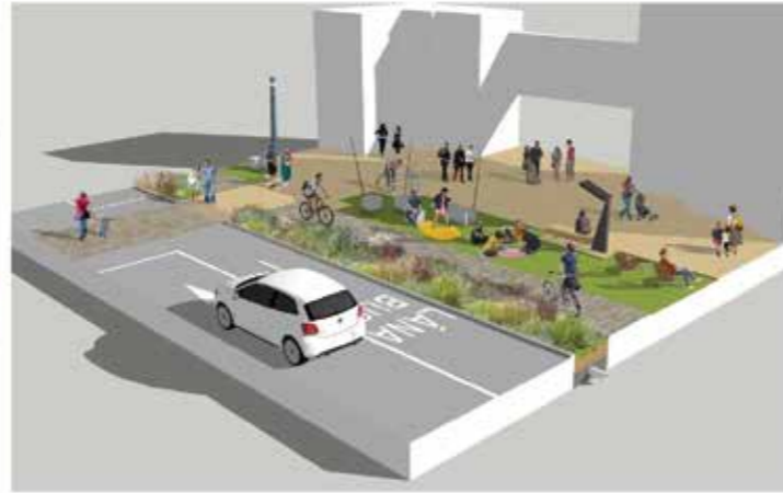
Extra wide footway, rain garden, amenity zone with play and smart furniture
