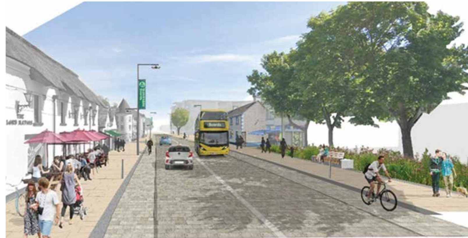
Main Street southern gateway as proposed, with traffic calming, enhanced pedestrian/cycle facilities and high-quality surfacing, street furniture and planting.
