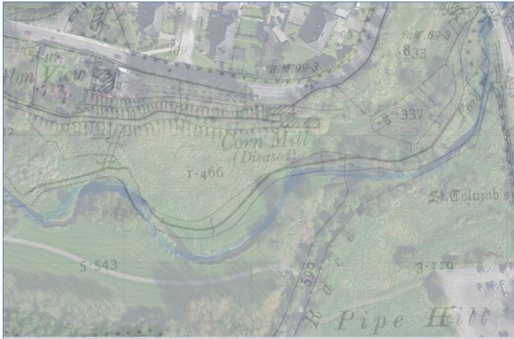
Fig. 4: Overlay of the Historic 25" map and the modern Geohive map onto the aerial premium image. River mapped in blue on the modern map.
