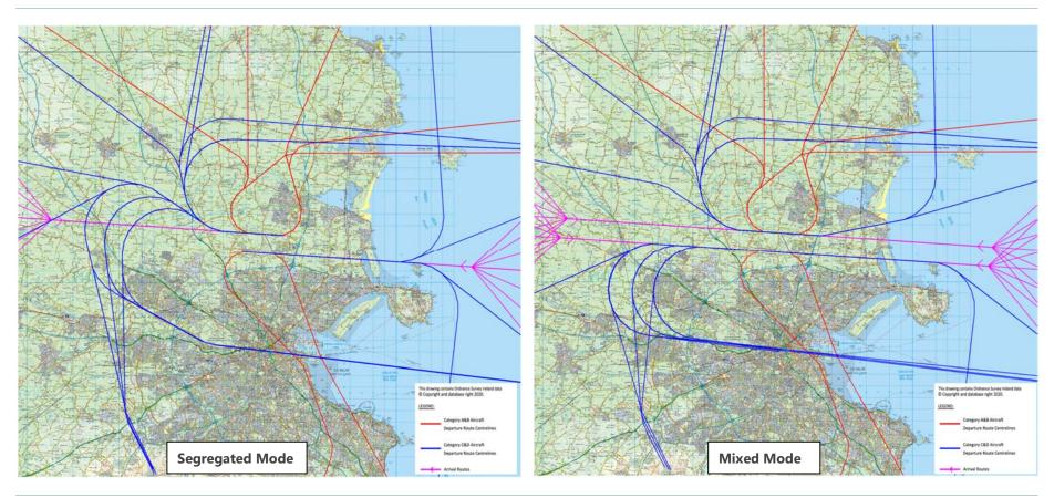
NOTE: The Irish Aviation Authority Air Navigation Services Provider has developed instrument flight procedures (IFPs) for all runways. Air Traffic Control operational procedures will accommodate whatever mode/time operation is decided upon for the runways.
