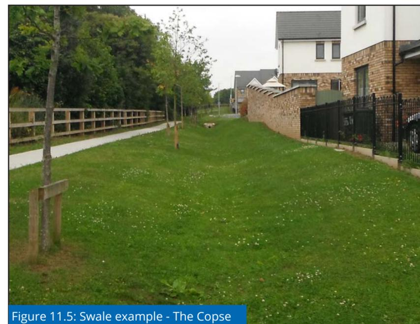
Figure 11.5: Swale example - The Copse
