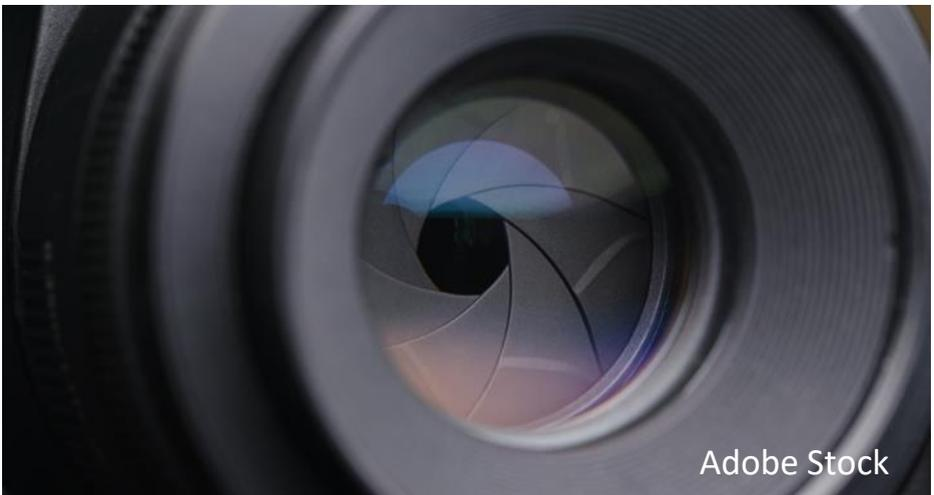
Take a look at the picture of a lens aperture above. Notice the adjustable blades that can move to adjust the size of the opening.
