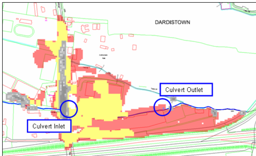
Figure 9-1 Mayne River flood extents at Swords Road for the current scenario, 30% blockage scenario and 70% blockage scenario
