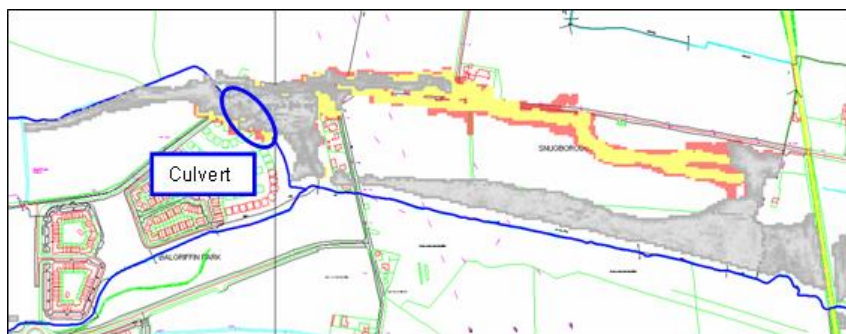
Figure 9-3 Cuckoo Stream flood extents at Wellfield Bridge for current, 30% and 70% blockage scenarios
