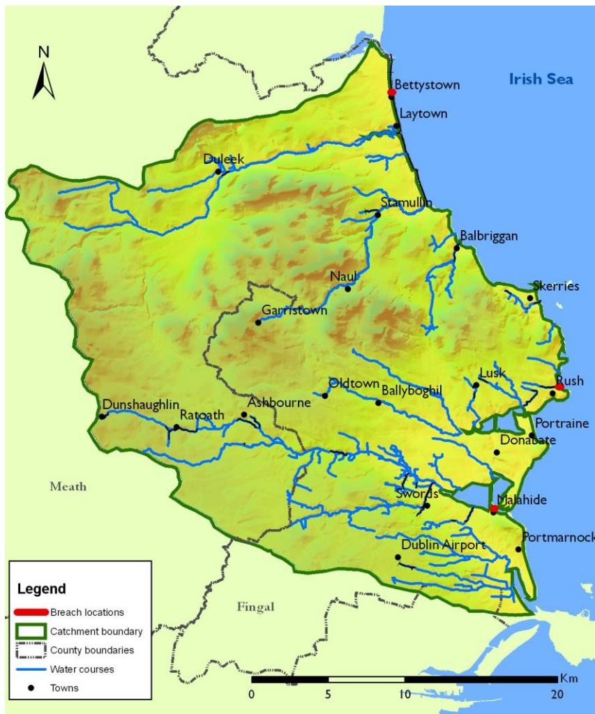
Figure 8-18 Breach locations in coastal defences
