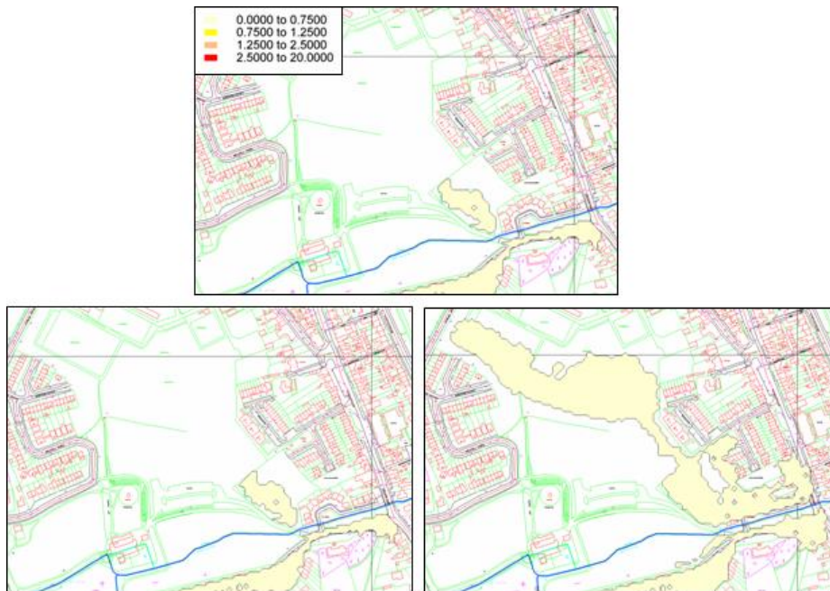
Figure 9-34 Mill Stream hazard maps at Holmpatrick Bridge for the current scenario (top), 30% blockage scenario (bottom left) and 70% blockage scenario (bottom right)
