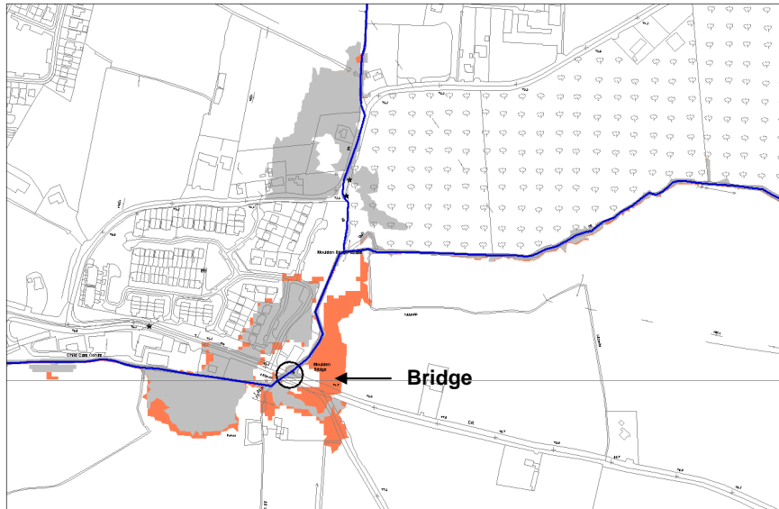
Figure 9-12 Broadmeadow River flood extents at Moulden Bridge for current scenario and 70% blockage scenario
