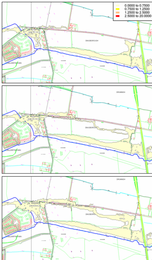
Figure 9-4 Cuckoo Stream hazard maps at Wellfield Bridge for the current scenario (top), 30% blockage scenario (middle) and 70% blockage scenario (bottom)
