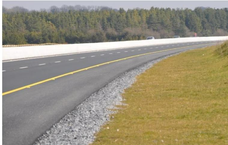
**Figure 6.7 Example Filter Drain**
