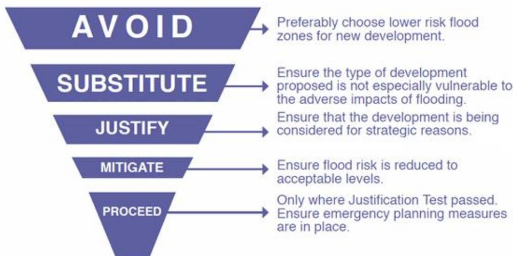
**Figure 2.2 Sequential Approach (The Guidelines)**
