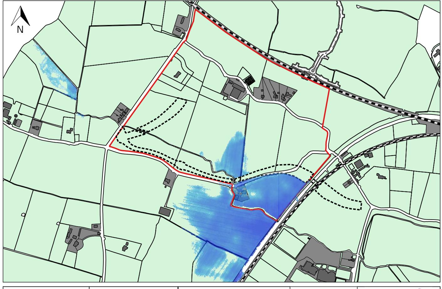
**Figure 2.7a Predicted flood extent for 100 and 1000 year flows with proposed road in place
