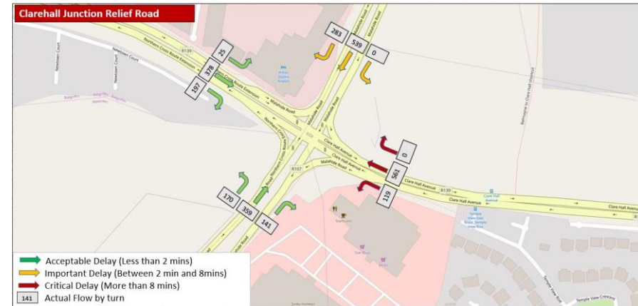
Figure 4.23 Congestion Clarehall Junction (with CJRR)
