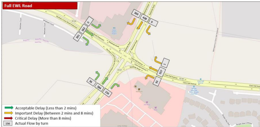
Figure 4.25 Congestion Level Clarehall Junction (Full EWLR)
