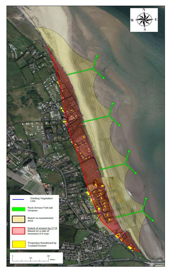
Figure 6.2: Layout and extent of a series of fish-tail groynes and beach renourishment areas that could be implemented along the Burrow to protect against erosion.
