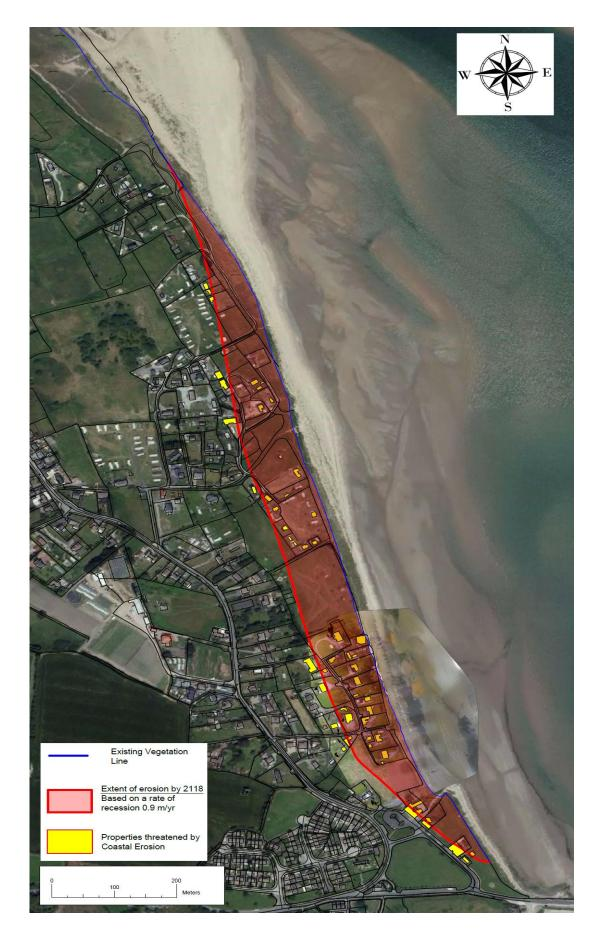
Figure 5.5: Extent of coastal erosion and properties at risk along the Burrow by 2118.
