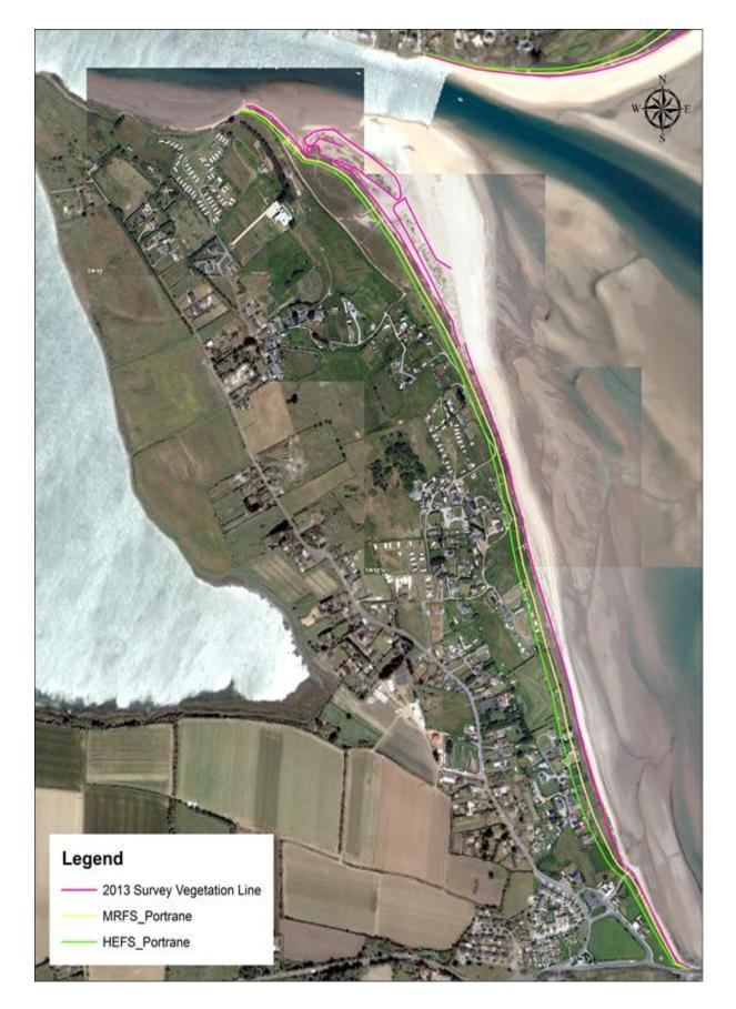
Figure 2.2: Position of the 2013 vegetation line and the 2100 MRFS and HEFS erosion lines.
