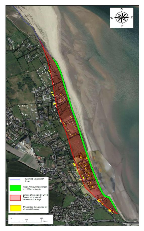
Figure 6.1: Layout and extent of a typical revetment structure (shown in green) that could be constructed along the Burrow to protect against erosion.
