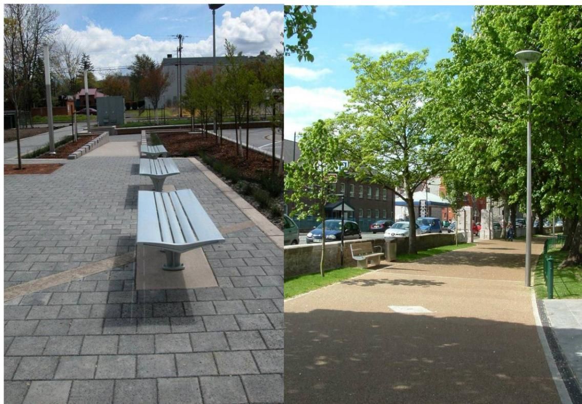
Fig. 6.12 – Surfaces: Quality granite finish (left) and gravel resin bond (right)
