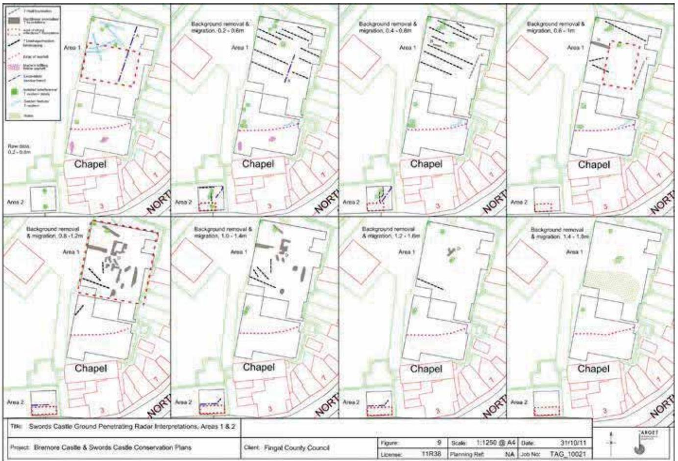
FIGURE 17: Interpretation of ground penetrating radar survey results
