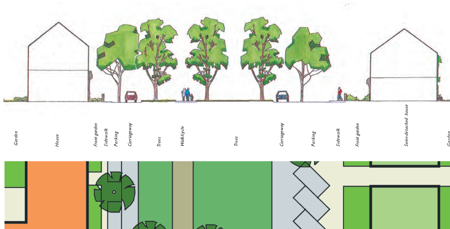
2.3.2.A Boulevard 1. Detailed plan and Section (41,5m wide)
