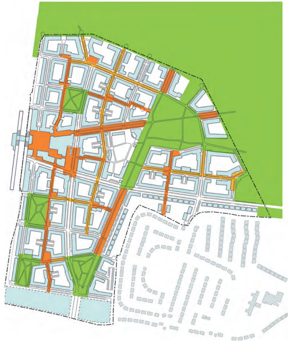
2.2.2.A Detailed plan pedestrian & cycle paths
