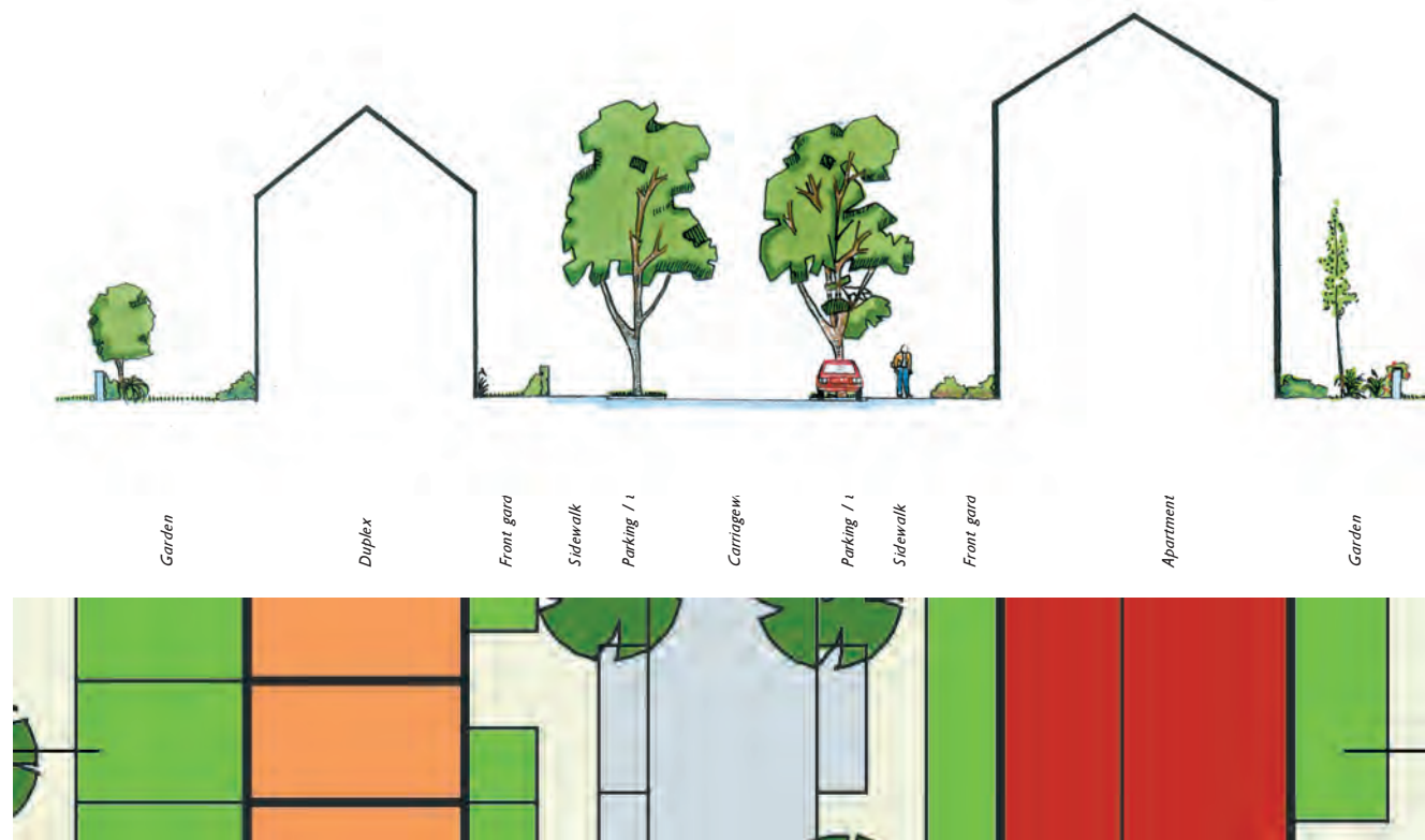
2.3.2.E Main street 2. Detailed plan and section (18m wide)
