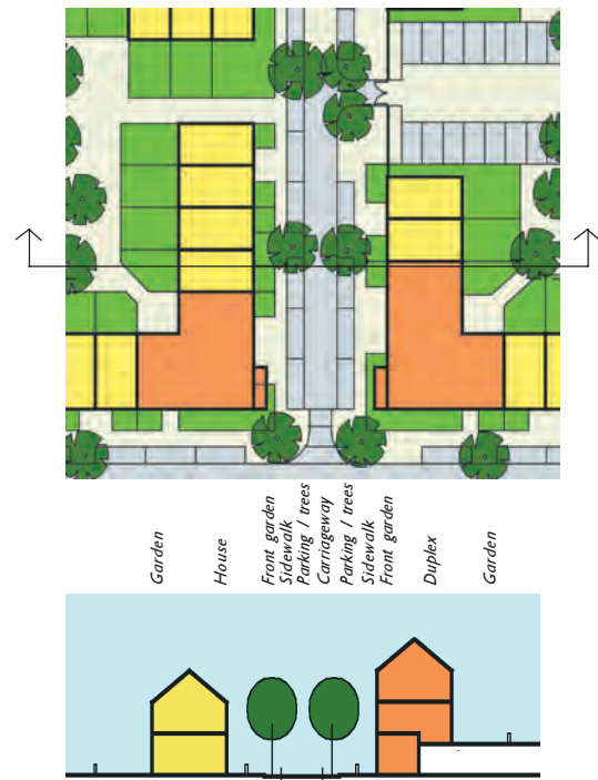
2.1.4.J Secondary street, plan & section
