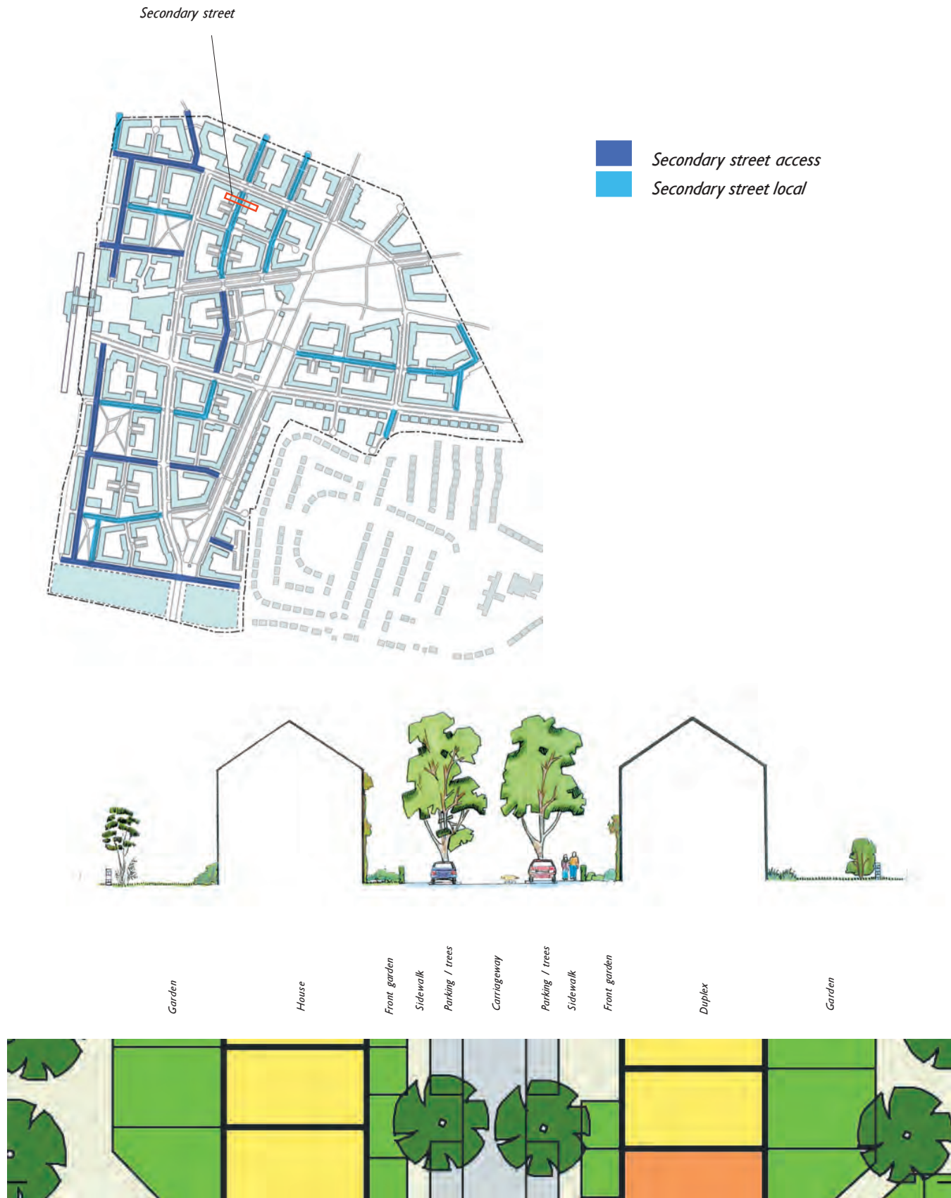
2.3.2.G Secondary streets. Detailed plan and section (16m wide)
