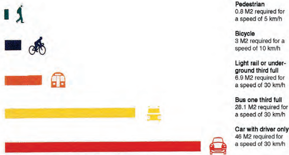
1.2.4.D Space required by one person for different modes at different speeds
