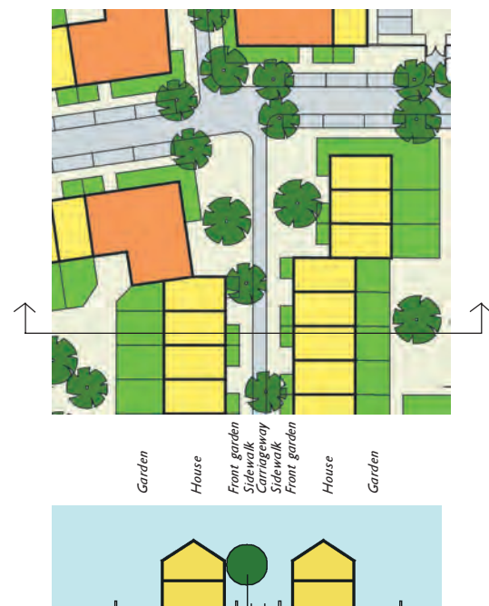
2.1.4.L Narrow street, plan & section
