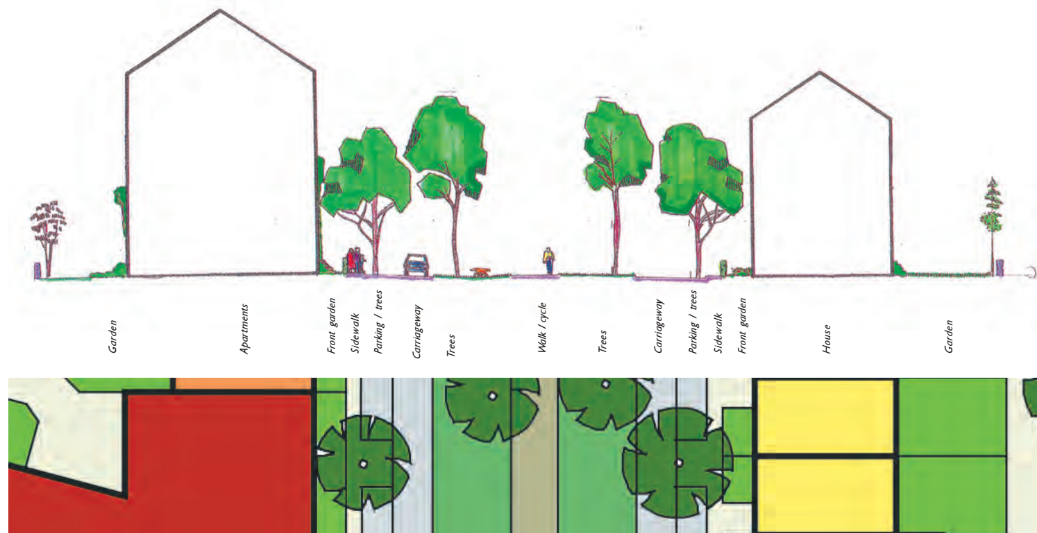
2.3.2.B Boulevard 2. Detailed plan and Section (28m wide)
