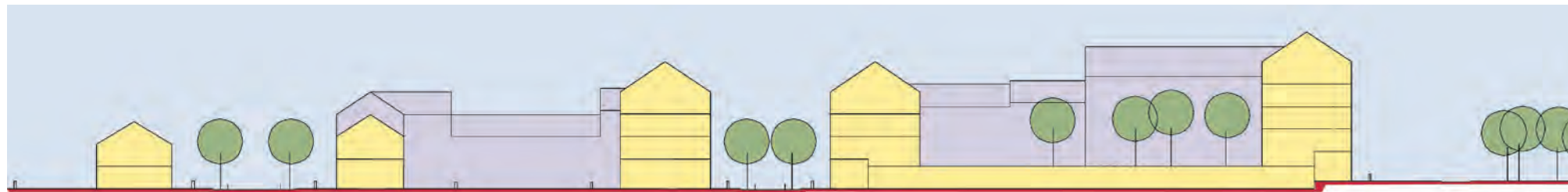
2.1.4.B Section indicating height to width relationship across streets and courtyards
