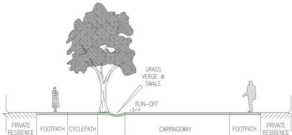
This SUDS cross-section provides a grass swale (wet or dry) on one side of footpaths and/or cycle-paths where a grass verge area exceeding 1.5m in width is adjacent. The swale will contain a grated manhole 'catch-pit' at its outfall which will enable each section to be connected to an overall surface water collection and distribution system.
