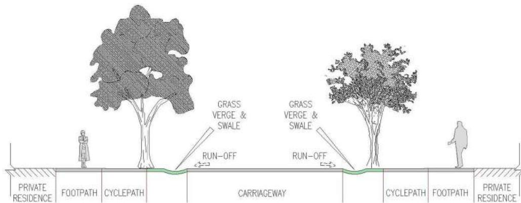
This SUDS cross-section provides road-side grass swales (wet or dry) on both sides of the reservation where grass verge areas exceeding 1.5m in width. Each swale will contain a grated manhole 'catch-pit' at the outfall which will enable each section to be connected to an overall surface water collection and distribution system.
