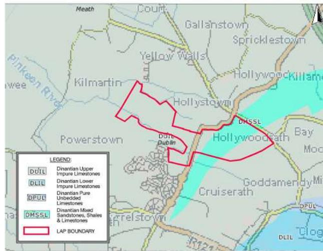
Figure 5 – GSI - Bedrock Mapping
