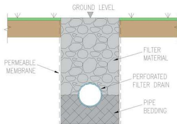
Filter Drain - Schematic
