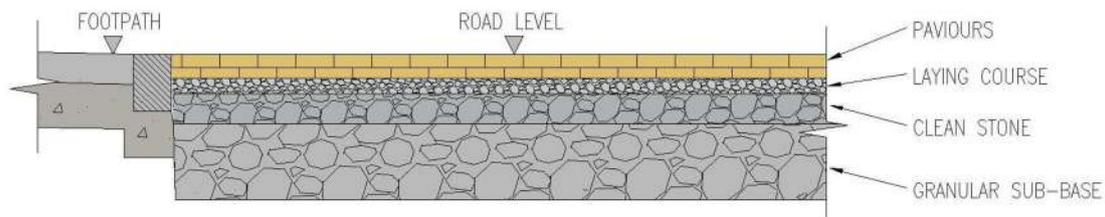
Permeable Paving - Schematic
