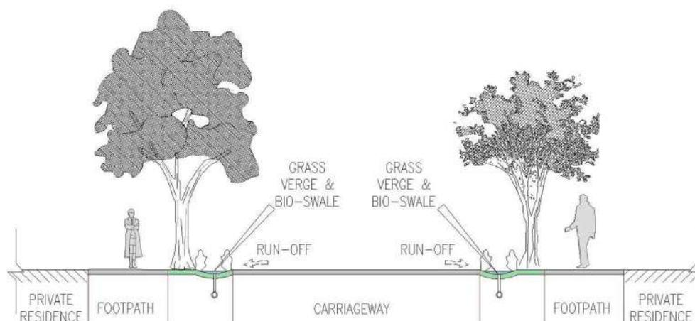
This SUDS drainage cross-section provides bio-retention swales (bio-swales) within planted verge areas adjacent to the road on each side. Bio-swales will be under-drained by filter drains and each section of bio-swale will be connected longitudinally
