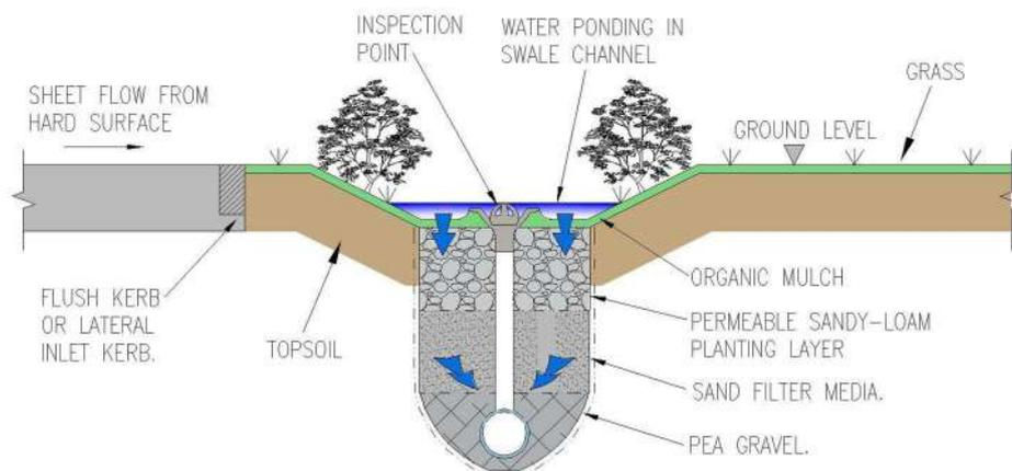
Bio-retention Swale - Schematic
