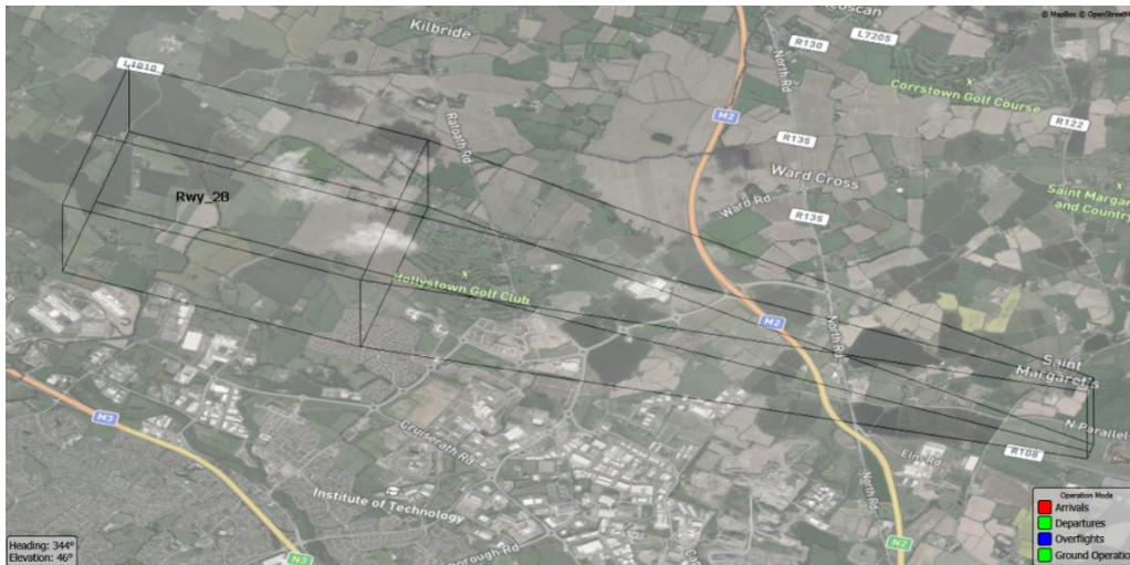
Figure 6 – Environmental Noise Corridor
