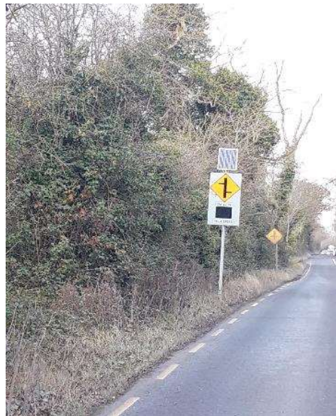
Newly installed Vehicle Activated Sign – Fieldstown R125/R122 Junction approach- Speed sign installed in November
